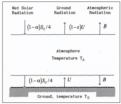
**FIGURE 2.6.** Single-layer model of the atmosphere. S is the Solar irradiance;  $\alpha$  is the albedo of the ground (0.05-0.2 for water-covered ground; 0.1-0.4 for bare ground; 0.1-0.25 for vegetated ground; 0.5-0.9 for snow-covered ground); U is the terrestrial radiation, of which a fraction  $(1-\varepsilon)$  penetrates directly through the atmosphere to space; B is the radiation emitted by the atmosphere (figure adapted from James (1994), see the list of books in section ii).
